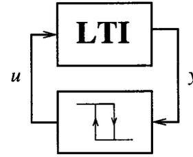
Fig. 1. Relay feedback system.
