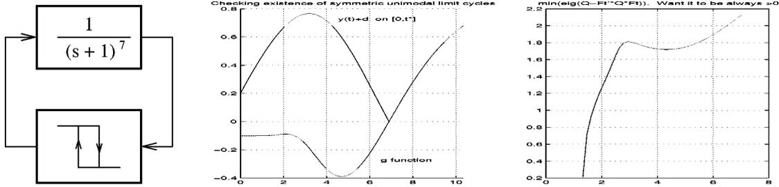
Fig. 11. System with relative degree 7.
