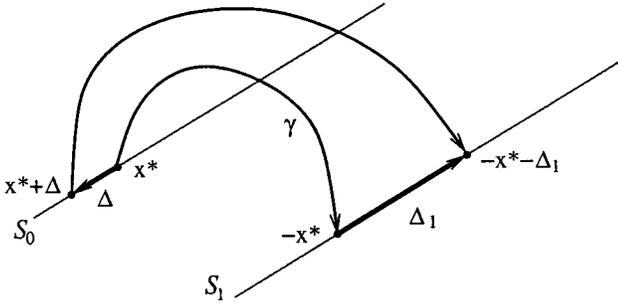
Fig. 5. Definition of a Poincaré map for a RFS.
