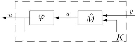
Fig. 6. Internal structure of the finite state stabilizing controller  $K$ .
