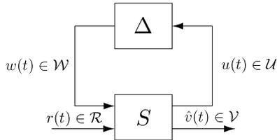
Fig. 7. Setup for the “small gain” theorem.
