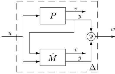
Fig. 4. Approximation error  $\Delta$  of  $P$  and  $\hat{M}$ .
