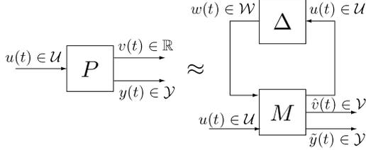
Fig. 3. Plant  $P$ , its DFM approximation  $M$ , and approximation error  $\Delta$ .
